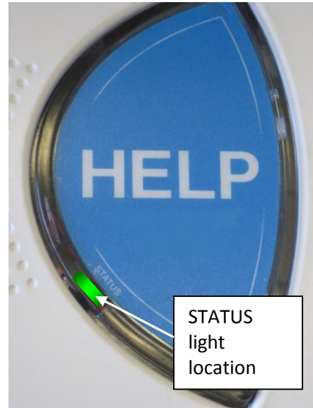
Figure 10. Status Light Detail
